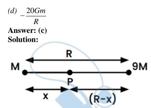
Let gravitational field at point P is zero. Which is situated at distance x from mass m.
